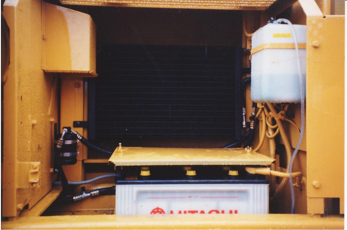
Condenser with drier and hoses in place.
